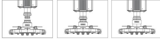
1. Align the 6 ball bearings on the wheel QR with the 6 notches on the base QR mount.
